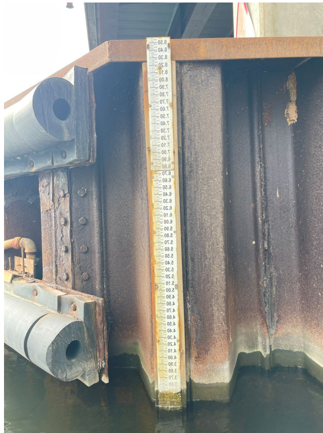
Photograph 8: USGS staff gauge in good condition.
